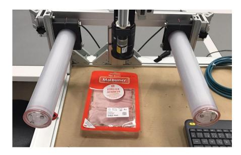
Versatile set-up with high-resolution camera and large field of view
